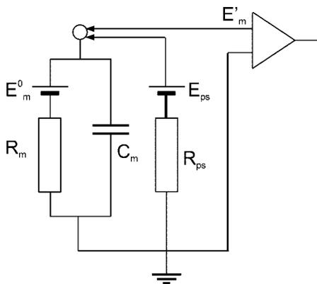
FIG. 6. Circuit diagram of patch-clamp recordings that includes the shunt through the seal between the pipette and membrane. Cell is presented by the whole cell resistance ( $R_m$ ), capacitance ( $C_m$ ), and the cell equilibrium potential ( $E_m^0$ ) that corresponds to the membrane potential of the intact cell. The seal contact is presented by shunt resistance ( $R_{ps}$ ) and the liquid junction potential between the pipette and extracellular solutions ( $E_{ps}$ ).
